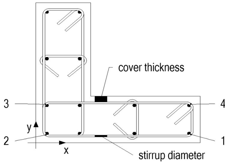
Fig. 8. Schematic diagram of the stirrup coordinate calculation
