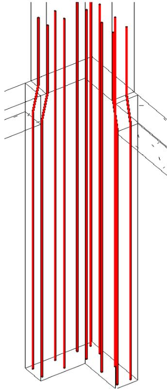
Fig. 7. 3D view of longitudinal rebar of L-column
