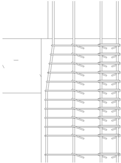
**Fig. 9. Side view of the stirrup in the variable section area of the column**
