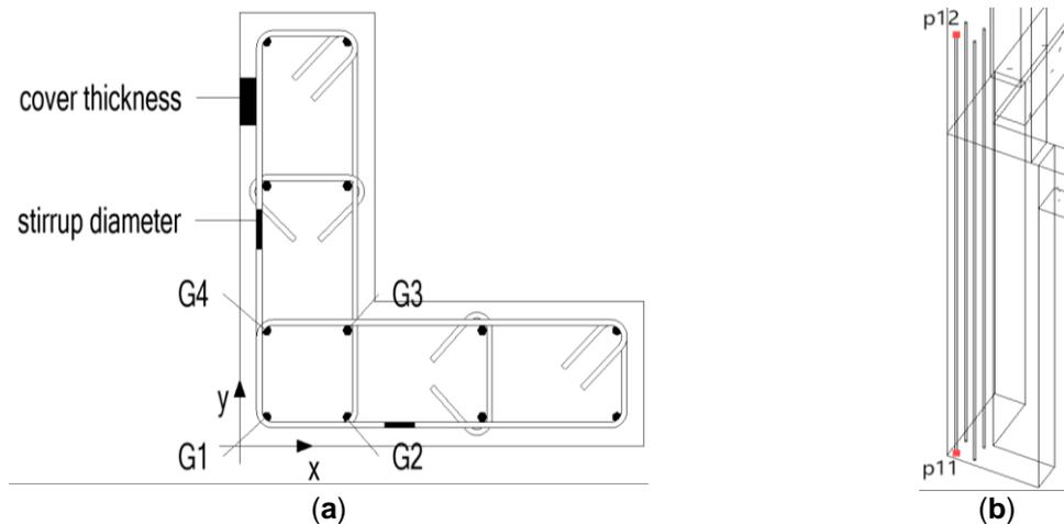
Fig. 4. (a) Schematic diagram of center longitudinal rebar; (b) Locating points for longitudinal rebar G1
