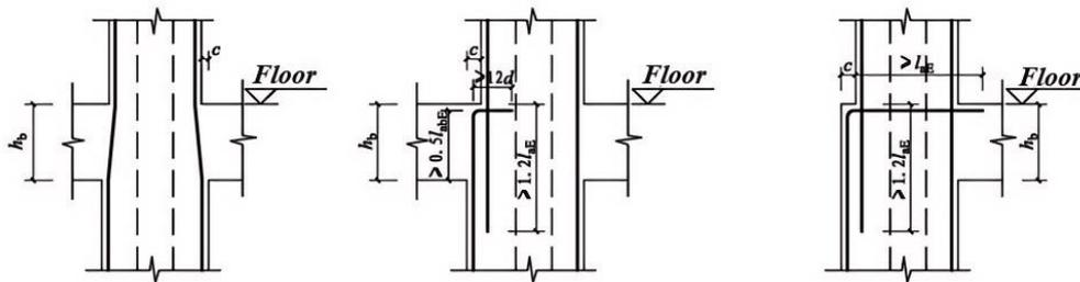
**Fig. 5. Longitudinal rebar at variable section of column**
