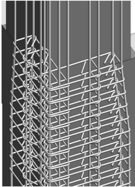
Fig. 10. L-column stirrup 3D (partial)
