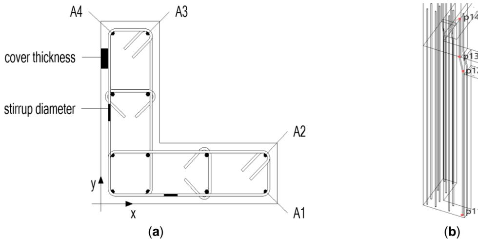
**Fig. 6. (a) Schematic diagram of column limb longitudinal rebar; (b) Locating points for longitudinal rebar A1**
