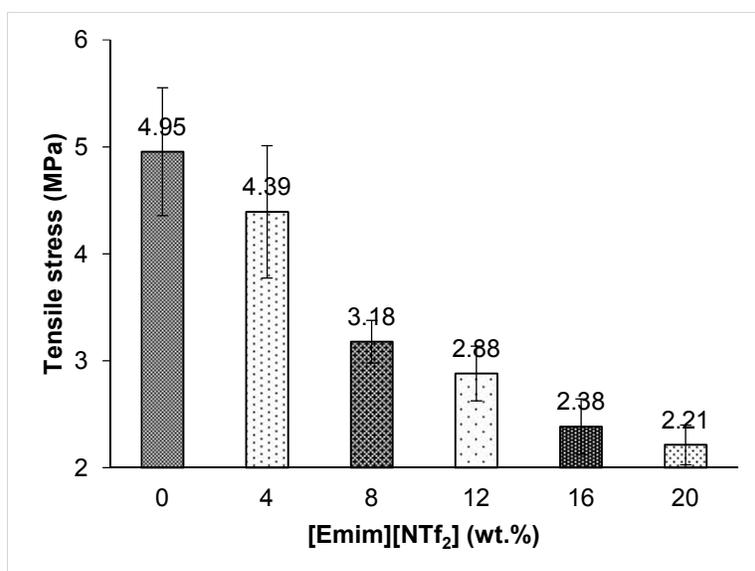
Fig. 1. Tensile stress of the HDPE/KCF biocomposites without and containing [Emim][NTf<sub>2</sub>]
