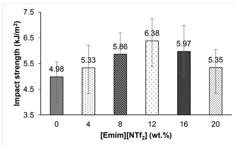
Fig. 4. Impact strength of the HDPE/KCF biocomposites without and containing [Emim][NTf<sub>2</sub>]
