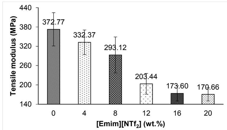
**Fig. 2. Tensile modulus of the HDPE/KCF biocomposites without and containing [Emim][NTf<sub>2</sub>]**
