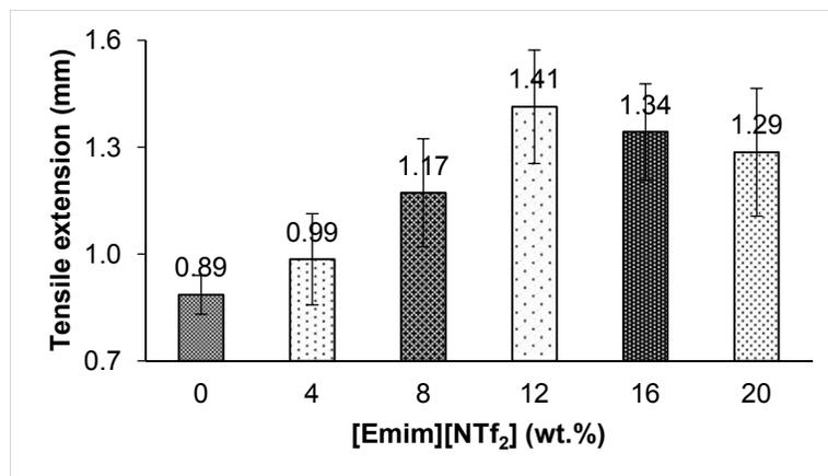
**Fig. 3. Tensile extension of the HDPE/KCF biocomposites without and containing [Emim][NTf<sub>2</sub>]**
